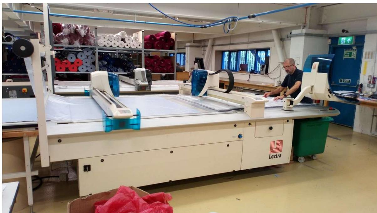
*Figure 22. The CNC cutting machine used at David Nieper.*
