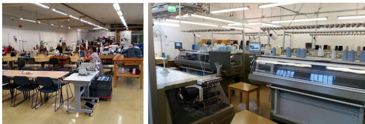
*Figure 6. Knitwear area. Linking machines (left) and knitting machines (right).*
